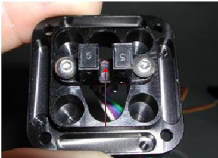
**Figure 10:** Close-up view of the optical homing sensor in the housing assembly.
