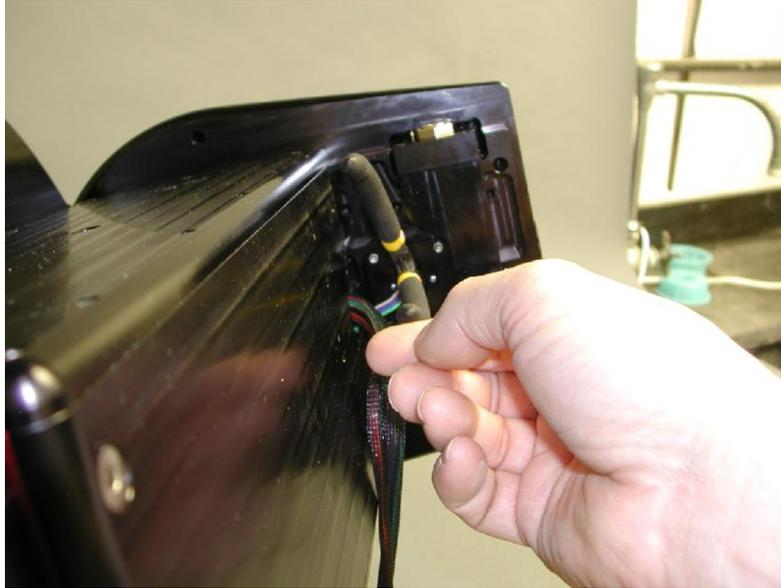
**Figure 9:** Use outward pressure on the needle nose pliers to carefully remove the sensor housing.
