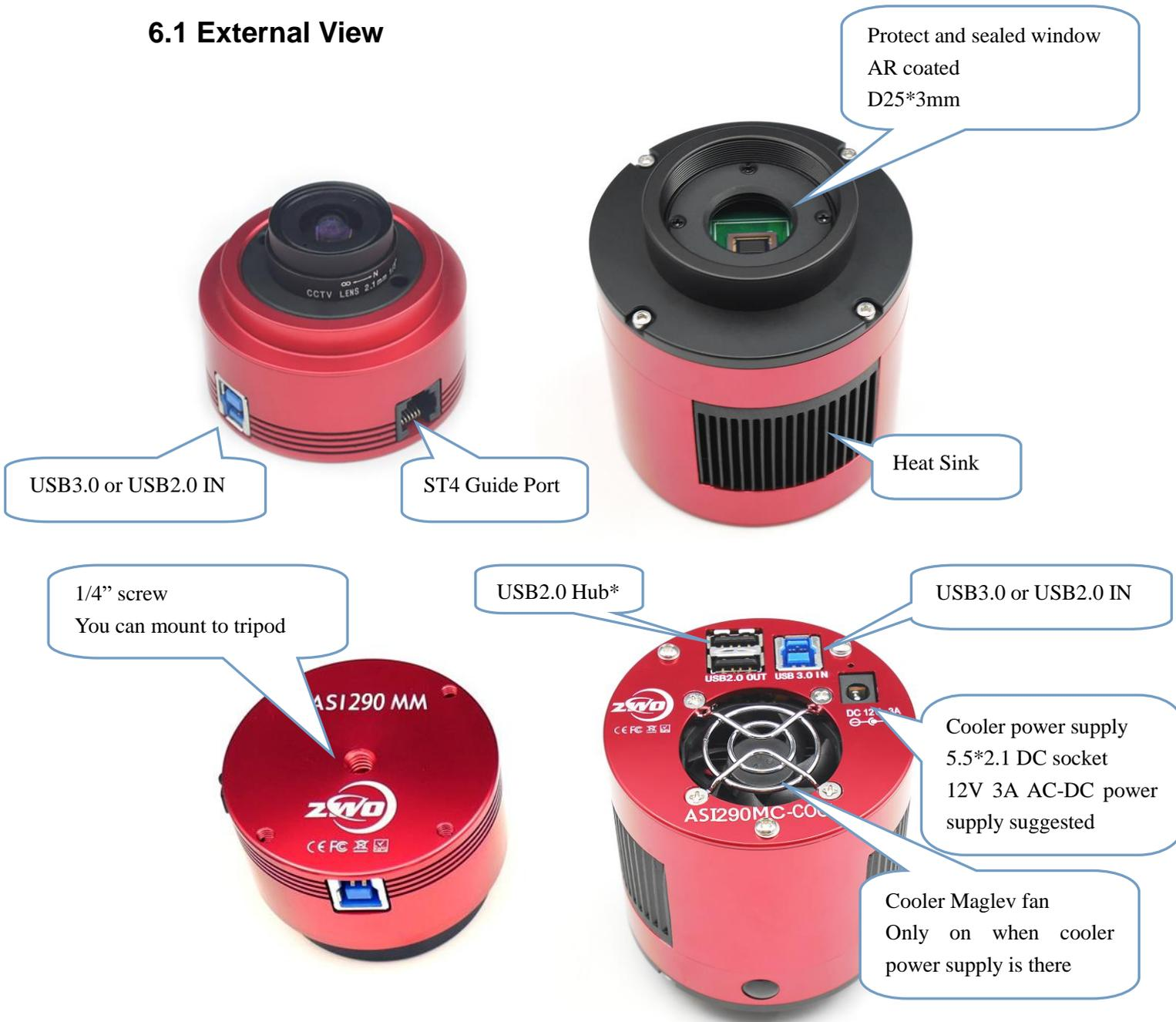
\*The first generation of cooled camera we used a ST4 port instead of USB2.0 hub
