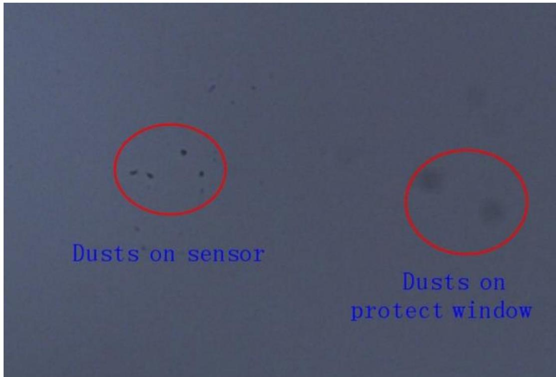
The big dim spot on the image (at right ) are the shadows of dust on the protect window.
